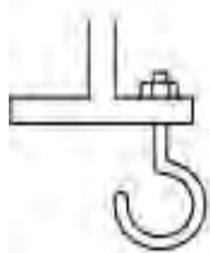
HOOK OR EYE BOLT THROUGH HOLE IN BEAM
